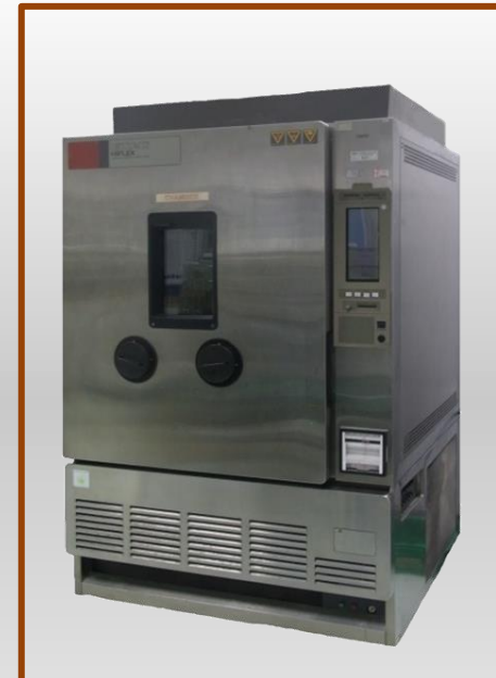
Temperature and Humidifier Chamber
